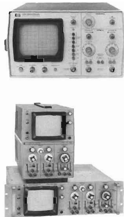
Figure 2. Representative Hewlett-Packard nonplug-in oscilloscopes.
